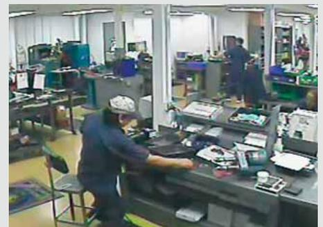
Once the subassembly is complete, the sections move on to the assembly area where by the demand of our stocking requirements they are completed. Once final assembly is complete each unit will be tested and new O-rings and tip protector installed.
